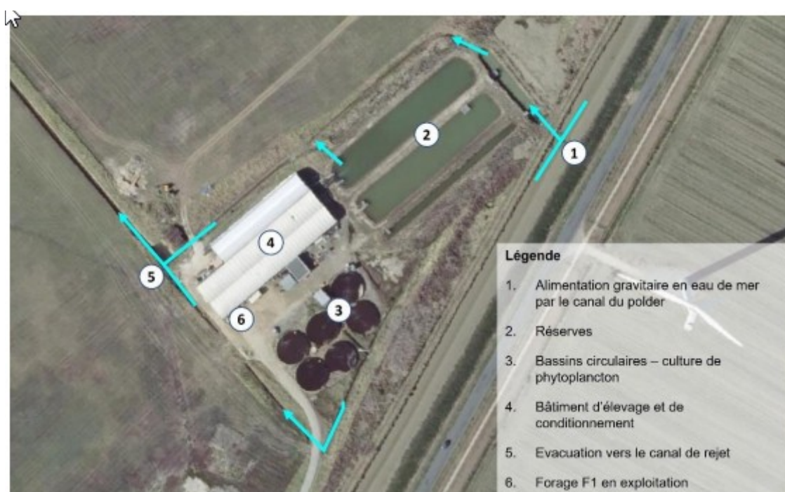
Installations existantes – Illustration extraite du dossier
